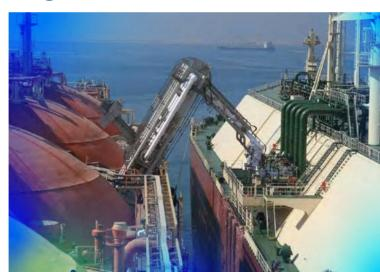
**DCMA-S** Double Counterweight Marine Arm Structure
