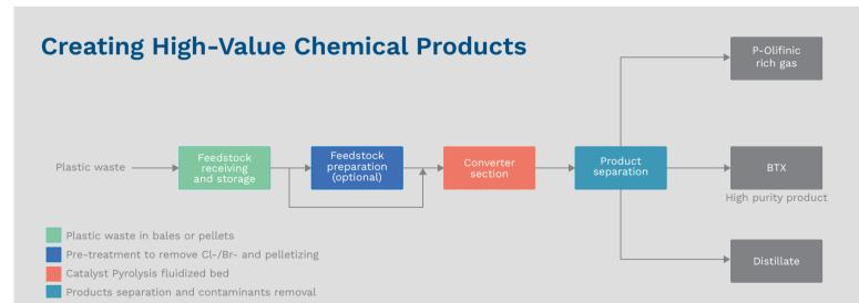
Plas-TCat technology consists of 4 sections: Receiver/ Storage, Pretreatment (optional), Catalytic pyrolysis (CP) and separation with post treatment. The CP is the core of the technology to aim to convert low-value plastic waste into high value chemical products. The technology is designed to overcome the limitations of traditional gasification and pyrolysis methods, offering an efficient, scalable solution for chemical recycling.
